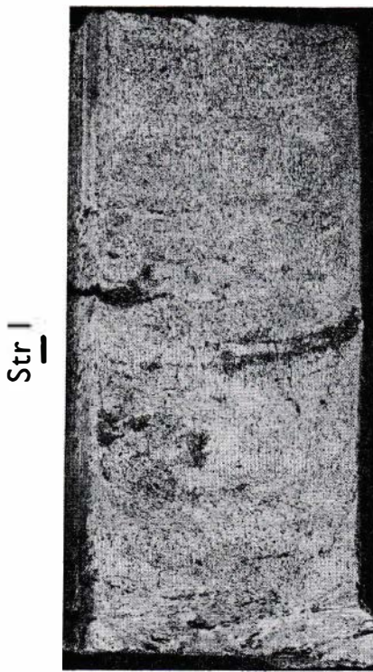
FIG. 36. Core E11, section Ph (photographed when dry). Pale grey moderately sandy to very sandy mud, showing pseudolamination. The well-defined near-horizontal structure (Str 1) is evidently a longitudinal section of a sandy relict burrow, with muddy faecal material in the centre. This structure indicates the origin of the fainter pseudolamination above and below. ( Actual size )
